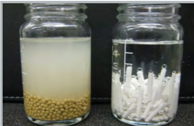
Figure 3 - Granular Desiccant vs. AMT in water
